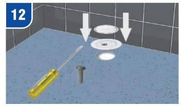
Once the floor coving is laid, screw into position the traps clamping ring using the bolts provided ensuring the inner cup and dip tube can still be removed. Fit the shower traps push on cover plate.
