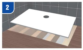
Remove the floor within the marked area to accept the DEC.
